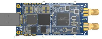
One problem with these SDRs is that they're really designed for experimentation on a bench. So output power is 10dBm (10mW) at best. actually measured one and for most of the frequency coverage it's hovering around
