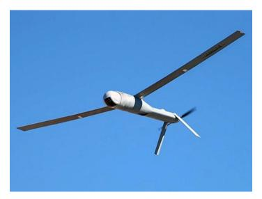
Furthermore, these air-launched drones are shot from tubes, so you can't have antennas hanging out, at least initially. Our command-and-control (C2) antenna operates in S-band (think 2.4GHz WiFi), and it's on a spring-loaded hinge. But the payload requirement is for transmissions somewhere in the military UHF band.
