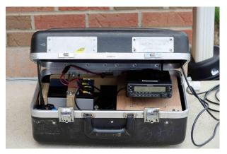
lesson the hard way at my first Market-to-Market relay. It's connected to the car via a battery isolator in case the car battery has issues) but I also typically have two HTs with spare batteries and a roll-up J pole as a backup antenna. There have been at least two occasions - Kettering Holiday at Home and ORRRC Marathon - where I've loaned out an HT to another station because their radio wasn't working for some reason.
