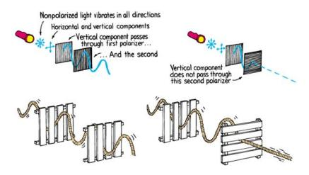
In electromagnetics, there is a concept known as polarization. Polarization by definition is the direction that the electric (not magnetic) wave is "waving". There are three kinds of polarization—vertical, horizontal, and elliptical with circular being a special case of elliptical. Vertical polarization is when the electric wave is waving up and down. Circular polarization is when the electric field is twisting at a constant rate—sometimes vertical, sometimes horizontal, some-
